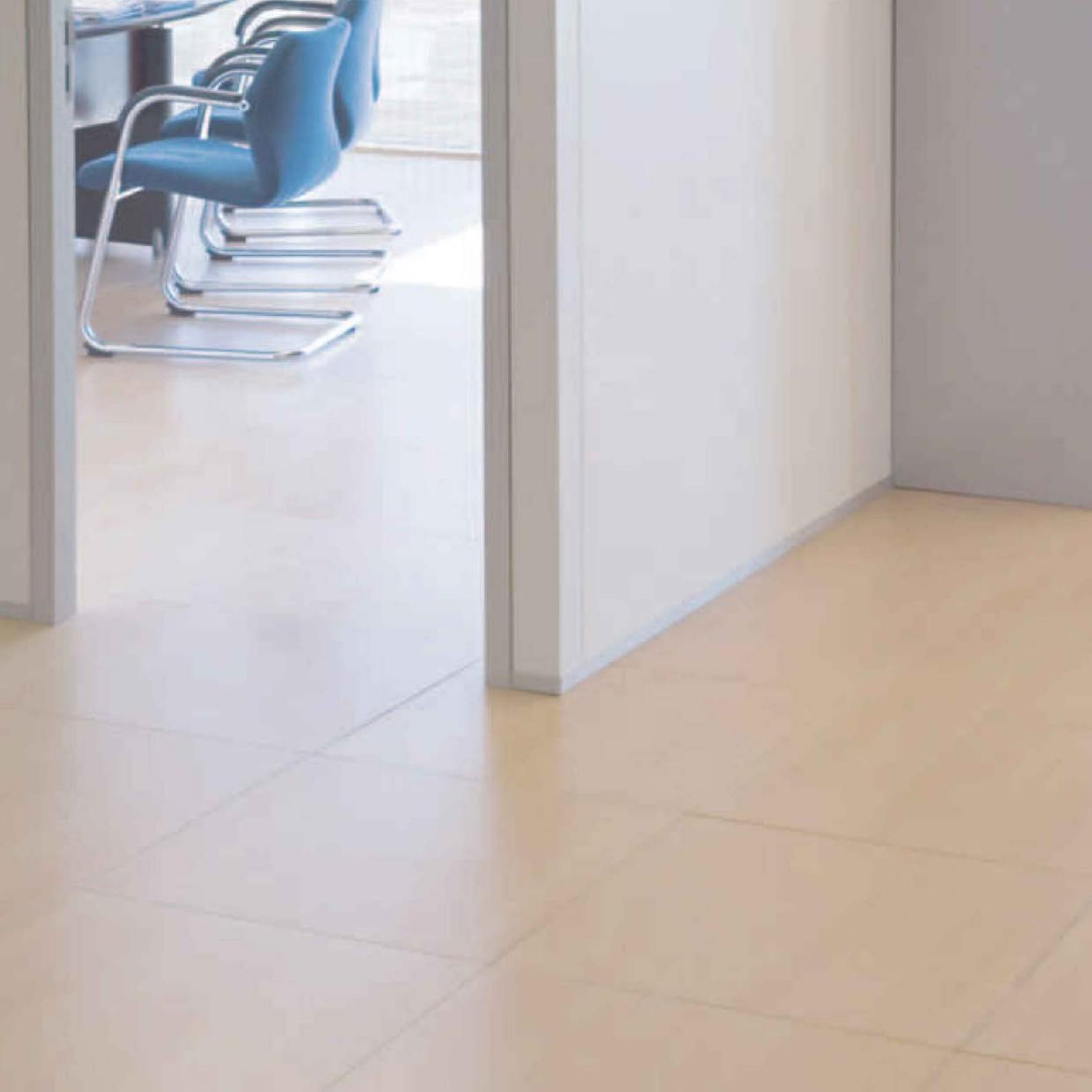
The system GAMAFLOR BANK is composed of tiles of 600x600mm, with chipboard core of high density \_between 700-720kg/m<sup>3</sup>, the bottom panel is a galvanized steel tray of 0.5mm with PVC edge. The top panel can be any floor covering.
